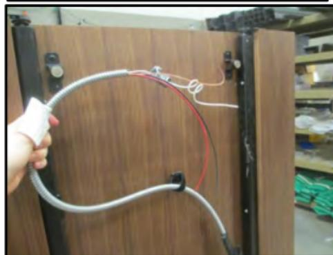
Step (3): Use the hardwires to connect to an electrical output through the end of the base
